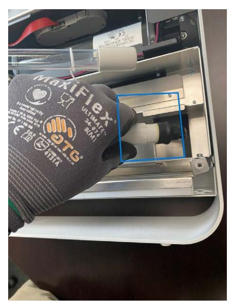
Connect the new optic to the optic harness cable.
