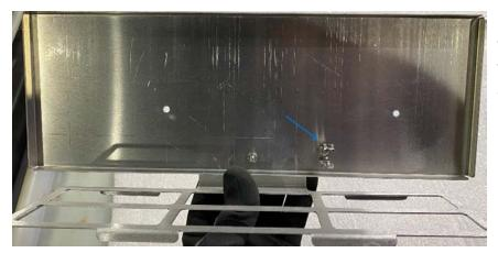
Note: Optional optic clip that might be located on the underside of the optic chamber cover.
