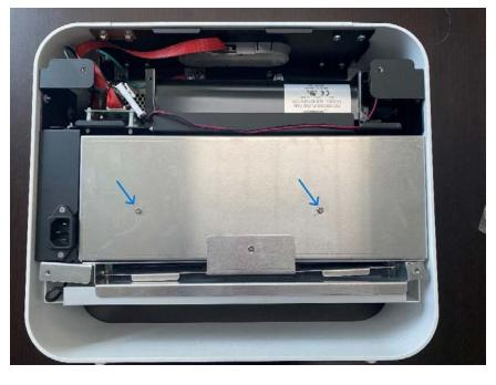
Loosen and remove the 2 screws shown to open the optic chamber.
