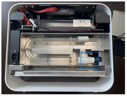
Locate where the optic is connected to the optic harness cable.
