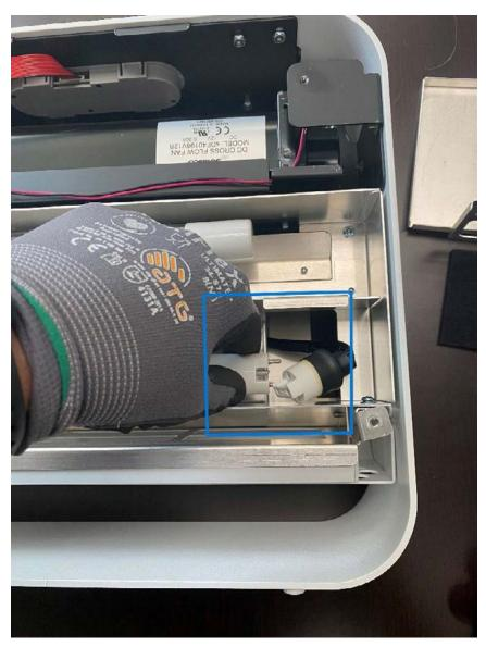
Disconnect the optic harness cable from the old optic.
