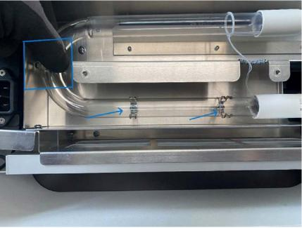
Lift one side of the optic from the optic clips. Gently remove the old optic and discard it safely.
